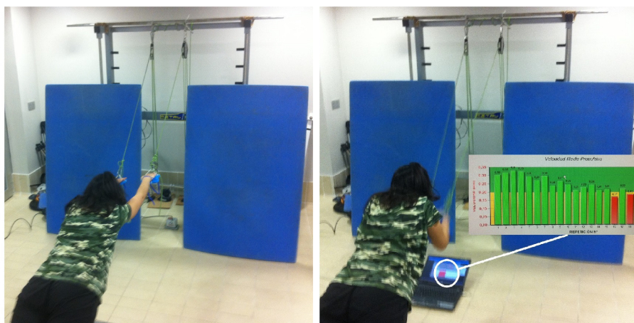
Fig. 1. The Smith Machine device showing both conditions (left: verbal feedback, right: visual feedback)
